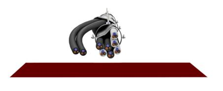
2. Wrap outlet cables over a length of ≥ 300 mm (with the coated side facing inwards).
