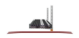
3. Fit the strips tightly in place (with the coated side facing inwards).
