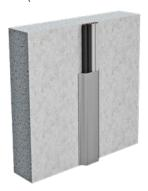
3. Arrange the next layer of strips with overlaps of  $\geq$  50 mm.
