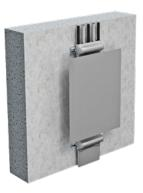
3. Fix the strips in place using steel band / wire.
