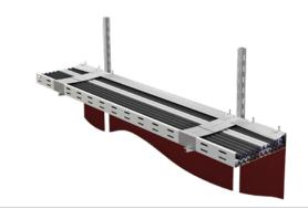
6. Fold the free end of the fire protection fabric over the cable tray and fix it in place circumferentially with steel bands/wires at a distance of ≤ 500 mm from each other (at least twice for each fabric section).
